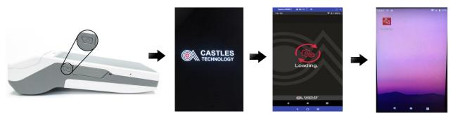
Press and hold the power button (on the left side of the terminal) until the screen lights up.
